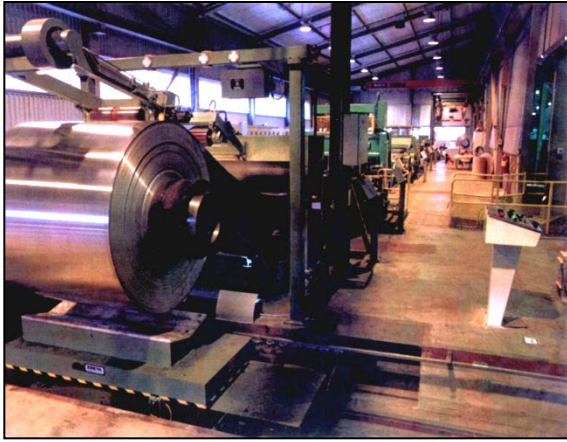
Entry section of tension level line
