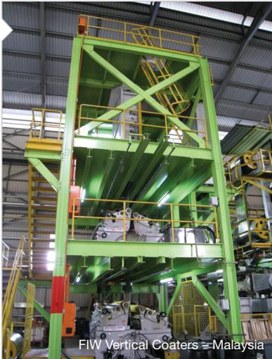
All Bronx Colour Coating lines can be configured for Satellite operation. Satellite reduces the line equipment required by removal of the cleaning and pretreatment sections. The pretreatment function is carried out at the exit end of a galvanising line, prior to the coil entering the Satellite Colour Coating Line.
