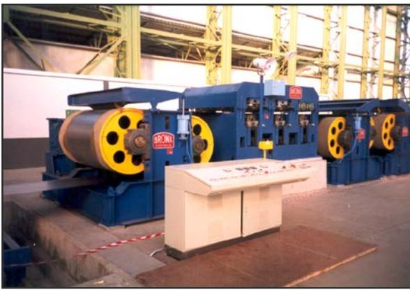
Tension leveller installed in a continuous galvanising line
