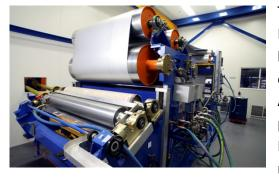
This machine is a modification of the S-Wrap Coater Machine. It provides all the characteristics and benefits of the S-Wrap Machine but also provides the excellent advantage of being a 'Quick Change Coater'. A Quick Change Coater is a machine that has two painting Heads for the top side of the strip. While one Head is painting the strip, the second Head is being made ready. When it is time to change paint colour,
