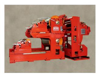
Whether a U-Wrap Machine is used or whether a C-Wrap Machine is used depends on the application area. The U-Wrap machine requires more space horizontally whereas the C-Wrap machine requires more space vertically. In both cases, the complete painting operation takes place in one room and this has good advantages for line manning and paint movement and storage logistics.
