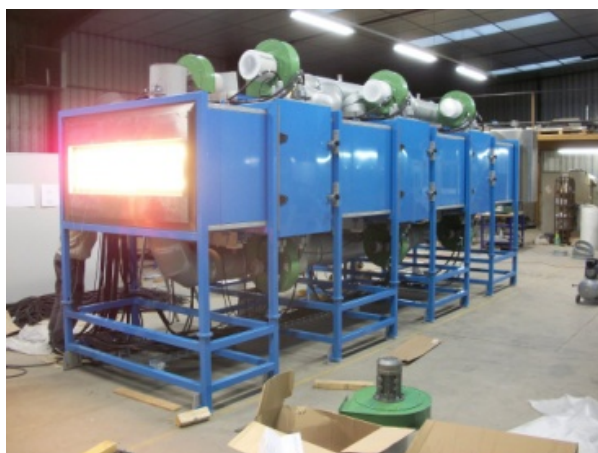
Figure 7.0: Electric Infrared Paint Curing Oven
