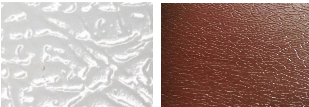
L to R: Embossed Metal Sample and Leathergrain Embossing
