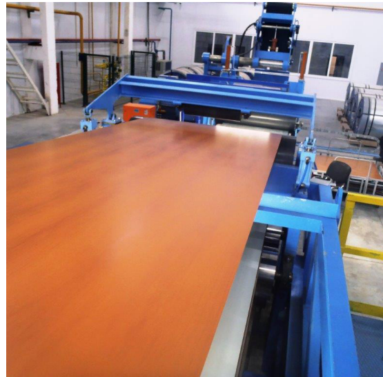
1250 Wide Line, Pattern Coating for Internal Wood Panelling
