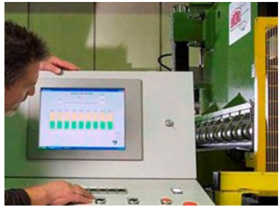
One of our technicians operating a leveller
