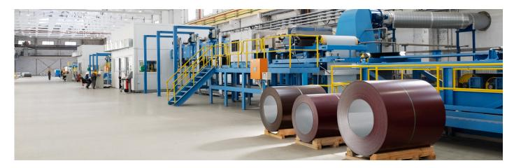
Bronx offers Colour Coating Lines customised to suit any business, from Compact Lines with a 10,000 tpa output to high-speed & high-capacity lines. Our lines are designed to apply either a superior quality three-coat system or an economical two-coat system.
